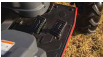
2. 2-range hydrostatic transmission (HST)
