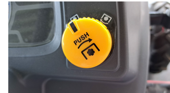
5. Independent electro-hydraulic PTO switch
